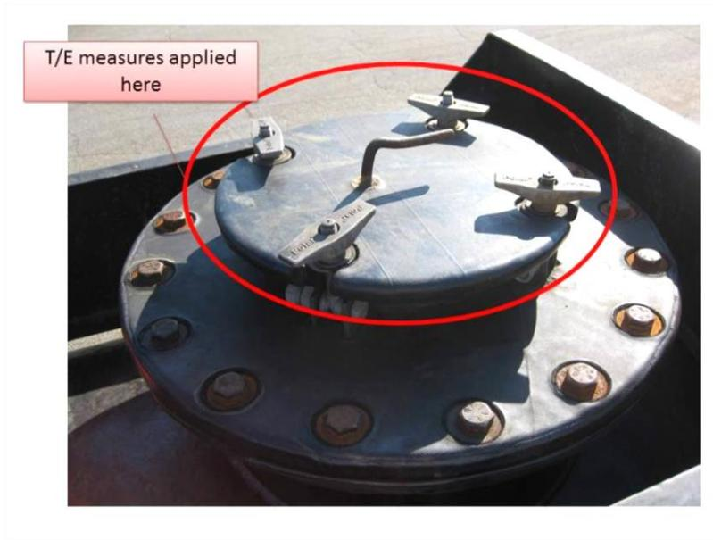
**Figure F1 - Common load point protected; torqued bolts are not.**
