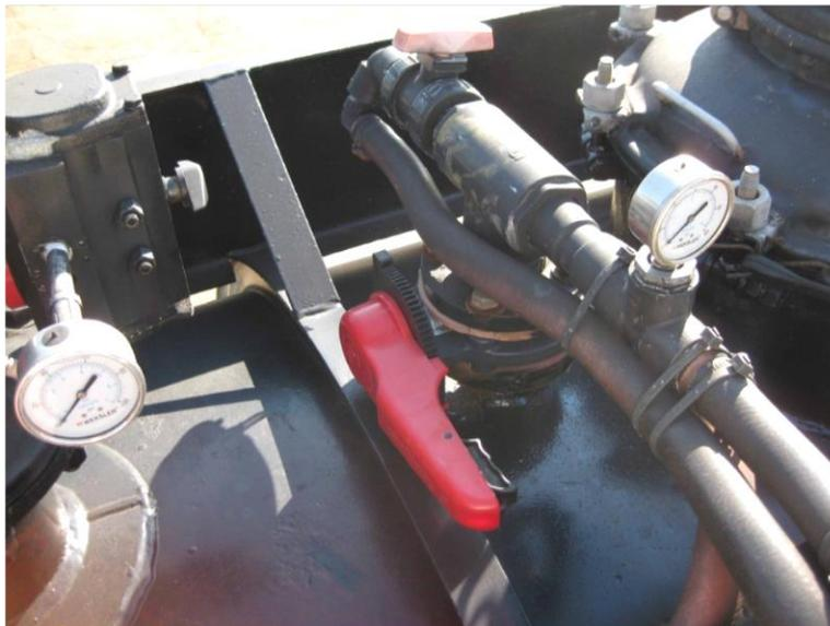
**Figure F8- Miscellaneous in-line plumbing not protected**
