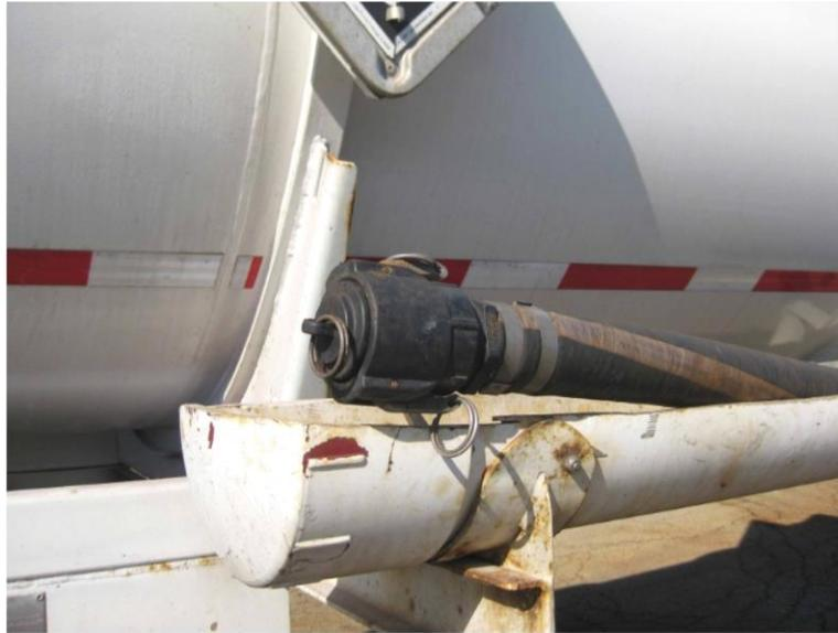
**Figure F111 – Off loading hose not protected**
