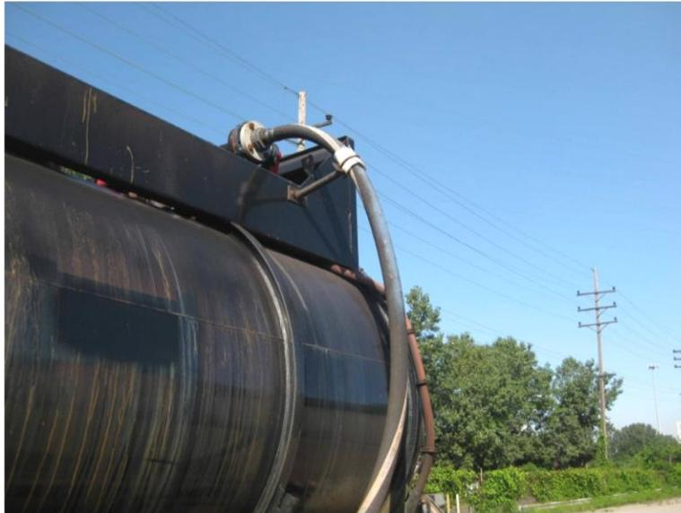
**Figure F7- Miscellaneous in-line plumbing not protected**
