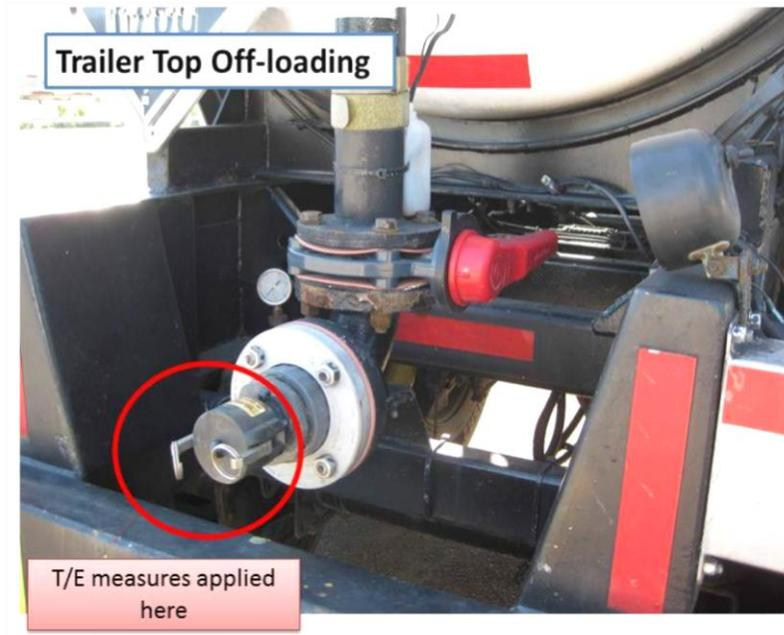
Figure F3- Common off-load point protected; torqued bolts and misc. air fittings are not.
