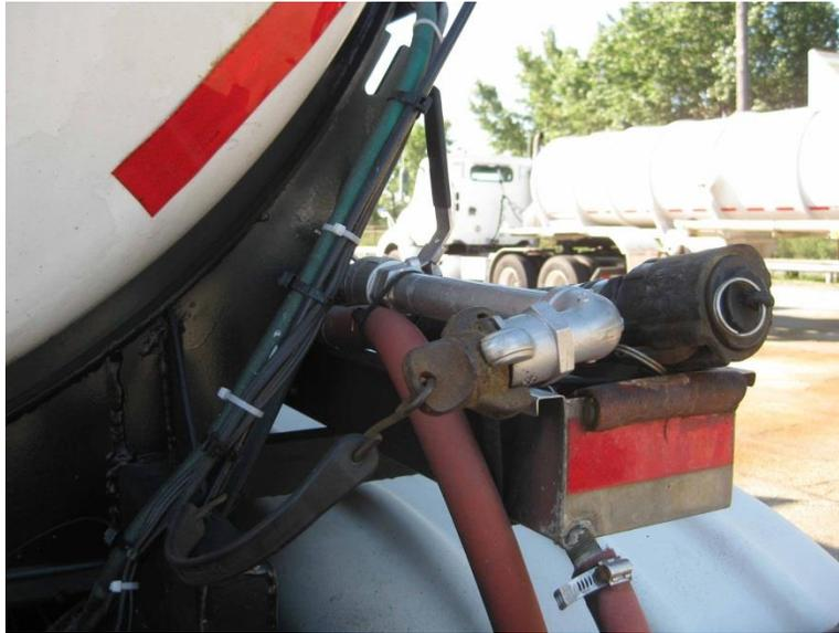
**Figure F5 - Air fittings and offloading hoses not protected**
